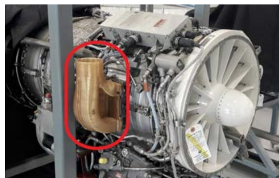
Functional bleed valve duct (circled) made with high-performance FDM thermoplastic.
